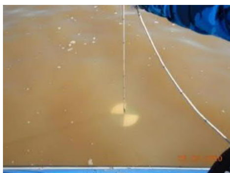
Figure 425 – Measuring transparency with the Secchi disk.
